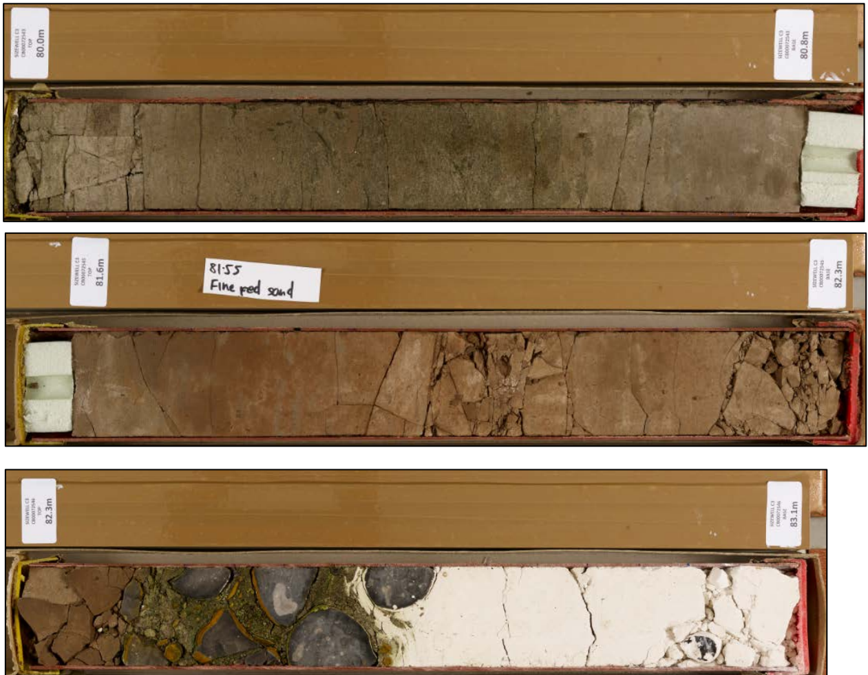
Figure 9-10: Lista Formation, Ormesby Clay Member. Pebble unit of OC1 in base photo, reddish unit of OC2 in middle photo and OC3 in top photo.
