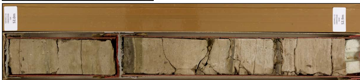
Figure 9-5: Wrabness Member in Sizewell C3 hole. Volcaniclastic layers are visible in the bottom picture and Harwich Stone Band with the dark central ash band in the top picture.
