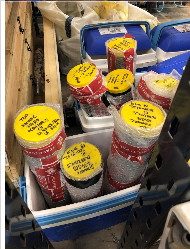
Sample is waxed again and then placed within a liner with end caps which are taped down. Bubble wrap is taped around the liner for extra transfer protection.
