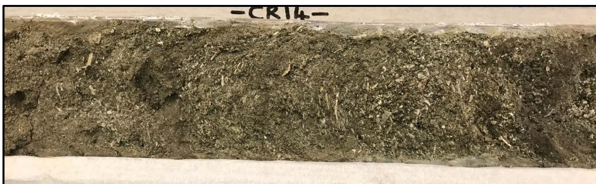
Figure 9-2: Red Crag Formation. Fine to coarse sand with abundant shell fragments.
