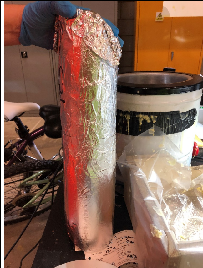
Sample is wrapped in cling film and then foil.
