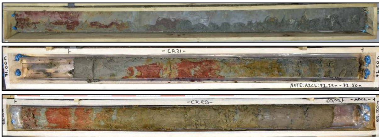
Figure 9-9: Upnor Formation. Top photograph is onshore, and the bottom two photographs are offshore. All show the mottled red top to the Upnor Formation at Sizewell
