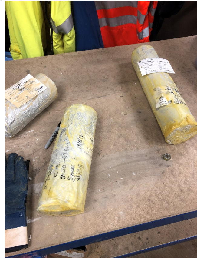
Sample is covered with wax and another label is placed.
