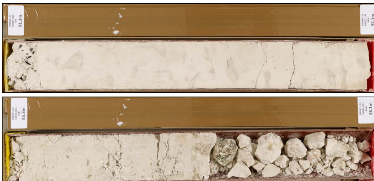
Figure 9-12: Weybourne Chalk. Glauconitic stained hardground visible in base photo, which is associated with the Catton Sponge.
