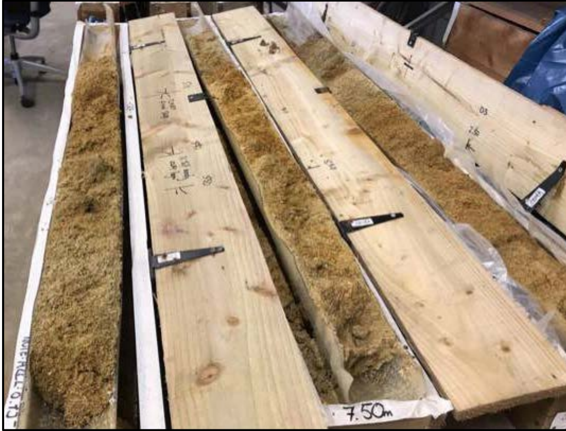
Figure 9-3: Coralline Crag Formation. Weakly cemented sand.
